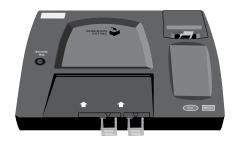
2. Plug the power cord into the rear of the scanner. Run the power cord through the grooves of the ballot box. Ensure that the power cord does not present a tripping hazard by taping it to the ballot box and floor, if necessary. Then plug it into a power outlet.
