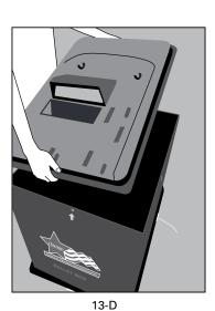
the ballot box and lock it into place. Make sure that the front of both of the ballot box and the scanner are on the same side, facing the same direction. Use the latch on the top of the ballot box to securely lock the ballot scanner into place. Secure the latch with a red tie seal. Secure the boxtop to the body of the box with red tie seals on all four sides. You must record the seal numbers on the Seal Accountability Form (Form 3).
