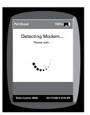
7. If Configuration Transmission was successful, press continue. Seal modem port door with a red seal. Place modem back into the red ballot scanner box. You must record the seal number on the Seal Accountability Form (Form 3).
